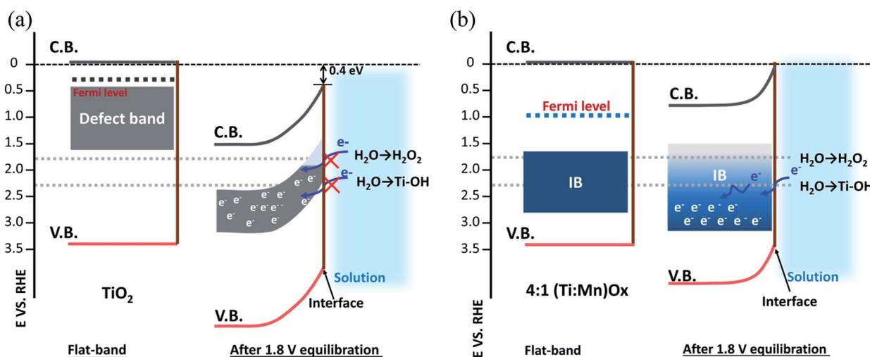
Fig. 5 Interfacial band energetics of semiconductive electrocatalysts. (a) “Leaky”  $\text{TiO}_2$  and (b) 4 : 1 (Ti,Mn) $\text{O}_x$  films. The left panel of each diagram was drawn under flat band conditions, and the right panel of each diagram was drawn where the electrode was poised at  $+1.8$   $V_{\text{RHE}}$  during water oxidation. Box height was drawn based on the estimated top edge of the  $\text{Ti}^{3+}$ -defect band or the  $\text{Mn}^{3+}$  intermediate band.
