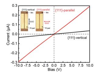
Fig. 4 I-V curves of the oriented TCNQ@Cu<sub>3</sub>(BTC)<sub>2</sub> thin films on polyimide substrates (Pt pads were 100  $\mu$ m apart from each other). Electrical measurements were carried out parallel to the {111} lattice plane ({111}-parallel) and vertical to the {111} lattice plane ({111}-vertical).
