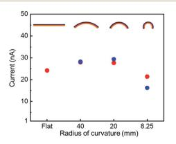
Fig. 5 Current as a function of bending radius of curvature at 10 V (blue circles: bending of a substrate perpendicular to the longitudinal direction (a-axis) of the underlying Cu(OH)<sub>2</sub> nanobelts. Red circles: bending of a substrate perpendicular to the short direction (c-axis) of the underlying Cu(OH)<sub>2</sub> nanobelts)
