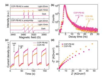
Fig. 4 (a) EPR curves for monitoring photo-excited electrons and holes. (b) Time-resolved transient PL decay spectra. (c) On-off photocurrent response under visible light or in the dark. (d) Electrochemical impedance spectroscopy Nyquist plots.
