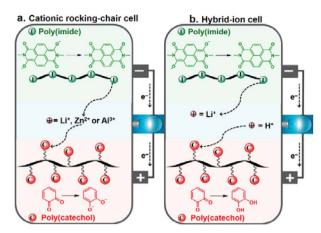
Scheme 1 Schematic of the working principle of the PI-PC full-cell during the discharge process in a cationic rocking-chair mode with Li<sup>+</sup>,  $Zn^{2+}$  or  $Al^{3+}$  (a), and hybrid-ion configuration with  $Li^+/H^+$  (b).
