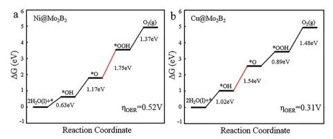
Fig. 4 The Gibbs free energy diagrams for the OER pathway of (a) Ni@Mo<sub>2</sub>B<sub>2</sub> and (b) Cu@Mo<sub>2</sub>B<sub>2</sub> at site I, where the red lines represent the most energy-consuming step of the OER.
