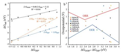
Fig. 6 (a) Scaling relationship between the  $\Delta G_{\text{OH}^*}$  and  $\Delta G_{\text{O}^*}$ ,  $\Delta G_{\text{OOH}^*}$  at site I. (b) Dual volcano plot for the OER and ORR for TM@Mo<sub>2</sub>B<sub>2</sub> at site I.
