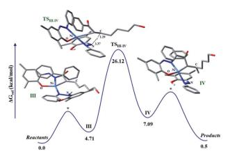
Fig. 2 Potential energy diagram of olefin hydrogenation of  $\alpha$ ,  $\beta$ unsaturated carbonyl via HAT (\* marked transition states are for illustration and were not determined). All hydrogens except chemically important ones have been removed for clarity.
