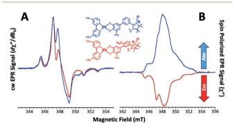
Fig. 4 X-band cw-EPR (A); 20 K; 2-MTHF, and TREPR (B); 20 K; 2-MTHF spectra for mPh-Pt (blue lines) and 6-Me-mPh-Pt (red lines). (A) Field modulation detected cw-EPR spectra of the ground states without light excitation. (B) Light-induced, spin-polarized TREPR spectra, extracted from time/field datasets 4 μs after the laser flash. Light excitation at 532 nm, concentrations  $\sim$ 0.5 mM. Abs = absorption, Em = emission.
