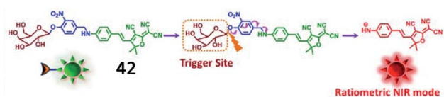
Fig. 32 Conceptual scheme of 42 when encountering \beta -galactosidase. Reprinted from ref. 129 with permission. Copyright 2017 Elsevier Ltd.
