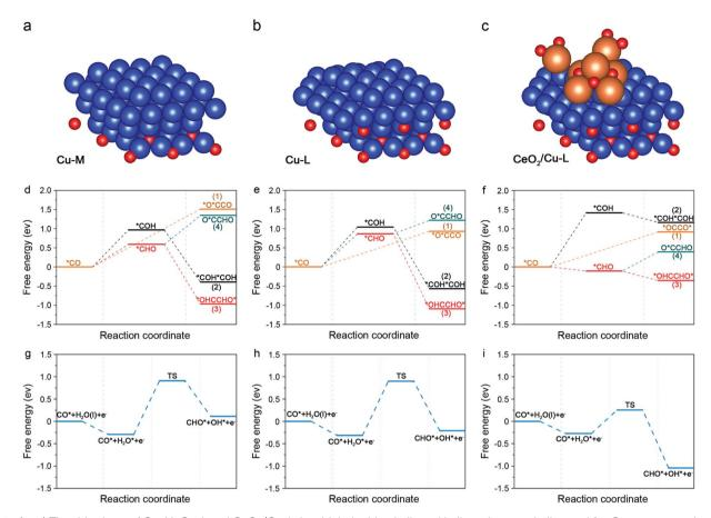
Fig. 4 (a–c) The side views of Cu–M, Cu–L and  $CeO_2/Cu$ –L, in which the blue balls, red balls and orange balls stand for Cu, oxygen, and carbon and hydrogen, respectively. (d–f) The reaction energy diagram for the  $CO_2/RR$  to describe the possible C–C coupling step from \*CO on Cu–M, Cu–L and  $CeO_2/Cu$ –L. (g–i) The reaction energy diagram for \*CO hydrogenation to \*COH on Cu–M, Cu–L and  $CeO_2/Cu$ –L, respectively.
