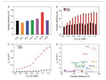
Fig. 2 (a and b) The average FEs of  $C_{2+}$  products at various potentials in 1 M KOH over CC0 and CC20, respectively. (c) The partial current density of C<sub>2+</sub> products at various potentials in 1 M KOH solution over CCO and CC20. (d) A comparison of the average FEs and the current density of C<sub>2+</sub> products on various reported catalysts and the literature sources are listed in the ESI (Table S1†).
