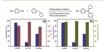
Fig. 5 (a) Conversions of the C-H arylation of 1c using Cd-MIX, Cd-TCA, and Cd-NPy<sub>3</sub> as catalysts and the excited state potentials of the three coordination polymers under optimal conditions. (b) Conversions of the C-H arylation of 1c using Cd-MIX, Cd-TCA, and Cd-NPy<sub>3</sub> as catalysts and the regioselectivity of N-benzyl arylation products under optimal conditions.
