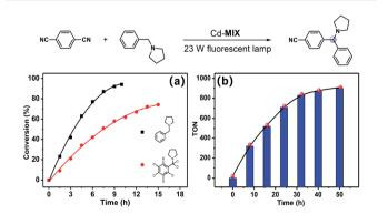
Fig. 4 (a) Kinetics curves of the C–H arylation using N-benzylpyrrolidine or N-((phenyl- $D_5$ )methyl- $D_2$ )pyrrolidine with 1,4-dicyanobenzene under optimal conditions. (b) The turnover number in scale-up experiments for C–H arylation of N-benzylpyrrolidine with 1,4-dicyanobenzene (0.64 g) within 50 h under optimal conditions.
