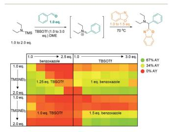
Scheme 5 Optimization via high-throughput screening: influence of 3 variables (benzoxazole, TBSOTf, and  $Et_2NTMS$  loading) on product yield. AY = assay yield, as determined by calibrated UPLC analysis (210 nm), using biphenyl as internal standard.
