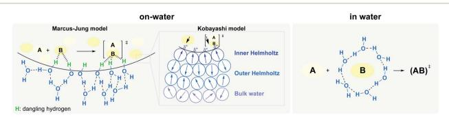
Fig. 5 Hydrogen bonding under heterogeneous (left) and homogeneous (right) conditions, at the oil—water interface, and Kobayashi's partial polarization approach (center).
