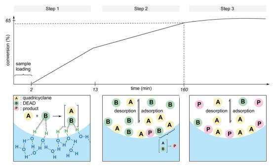
Fig. 6 Interface adsorption/desorption in micro-droplets.
