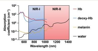
Fig. 7 Endogenous absorbers in the body within the NIR-I and -II regions. Adapted with permission from ref. 89, Copyright 2018 American Chemical Society.
