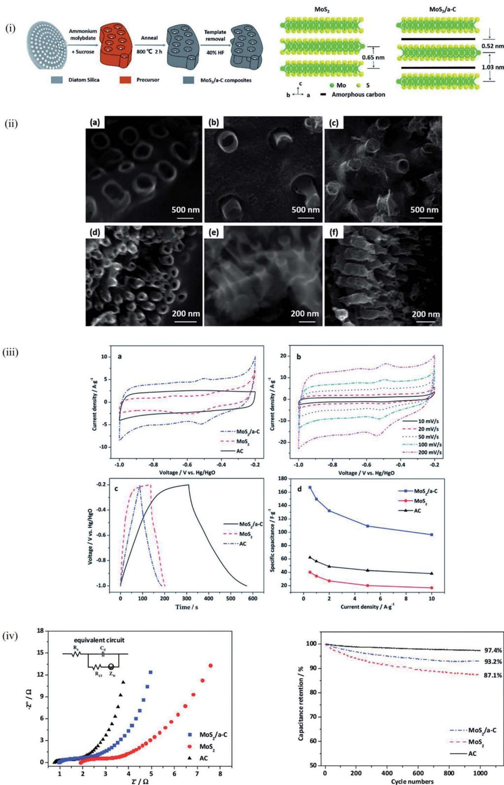
Fig. 9 MoS<sub>2</sub>/a-C composite prepared using DE templating (i) schematic representation of the synthesis process (ii) schematic representation of the microstructure of MoS<sub>2</sub> and MoS<sub>2</sub>/a-C composite (a and d) AC, (b and e) MoS<sub>2</sub>, and (c and f) MoS<sub>2</sub>/a-C composite (iii) and (iv) electrochemical performance of MoS<sub>2</sub>/a-C, MoS<sub>2</sub>, and AC.<sup>100</sup>
