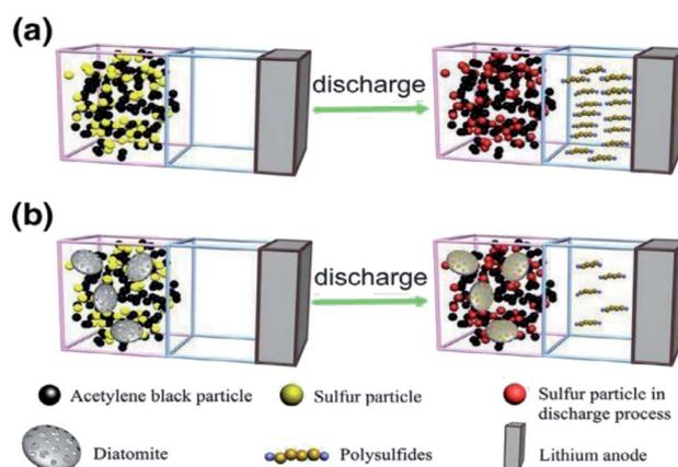
Fig. 6 Polysulfide suppression behaviour schematically illustrated for (a) sulfur electrode without DE (b) sulfur electrode with DE.<sup>83</sup>
