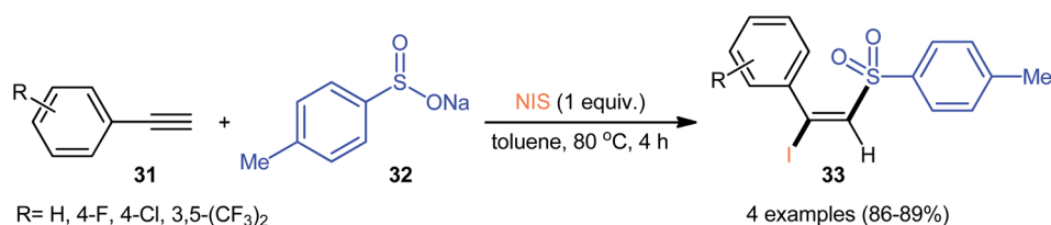
Scheme 14 Catalyst-free iodosulfonation of terminal aromatic alkynes 31 with sodium p -toluenesulfinate 32 and NIS.
