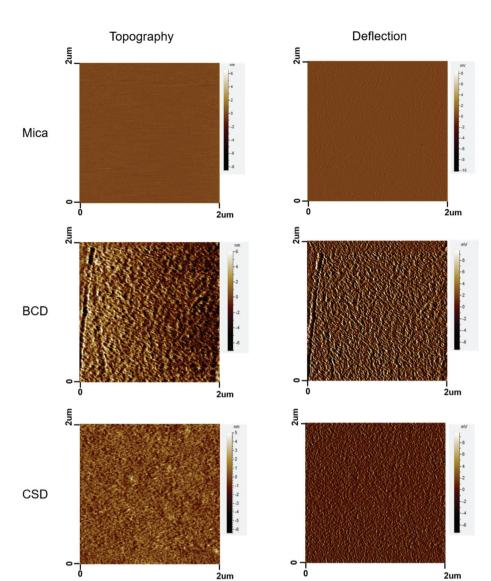
Fig. 3 AFM images of mica, BCD coated mica and CSD coated mica.
