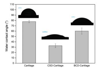
Fig. 4 Water contact angle of the cartilage surface and CSD or BCD coated cartilage surfaces.
