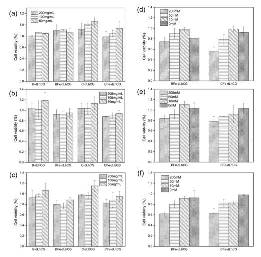
Fig. 8 WST-1 results based on different CSD or BCD concentration on (a) day 1, (b) day 4, (c) day 7 and WST-1 results based on different Fe<sup>3+</sup> concentration on (d) day 1, (e) day 4, (f) day 7.
