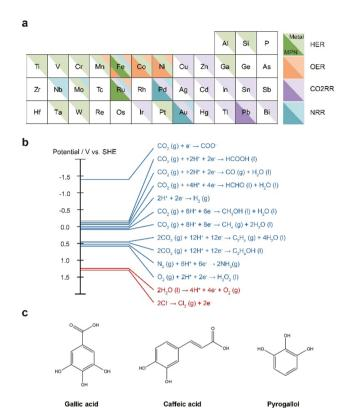
Fig. 8 (a) The periodic table summarizing the experimentally observed relationship between the main elements of catalysts and the preferred target electrochemical reactions. (b) Theoretical redox potential for various electrochemical reactions. (c) Various plant-derived polyphenolic molecules.
