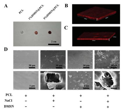
Fig. 1 Characterization of the DMSN@PCL scaffolds. (A) Images of the plain PCL and DMSN@PCL scaffolds (1% and 5% of DMSN); (B) confocal scanning of the DMSN@PCL scaffolds without NaCl ( $160 \times 160 \times 20 \mu m$ ) and (C) DMSN@PCL scaffolds with NaCl ( $1400 \times 1400 \times 86 \mu m$ ); (D) SEM images of PCL, PCL with NaCl, DMSN@PCL without NaCl, and DMSN@PCL with NaCl.
