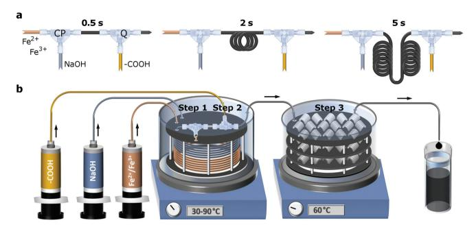
Fig. 1 Schematic of (a) precisely-timed quenching (Q) of particle growth after 0.5 s, 2 s and 5 s after initiation of co-precipitation (CP) and (b) multistage flow reactor to initiate co-precipitation (step 1), guenching and stabilisation (step 2, here after 0.5 s) and aging (step 3).
