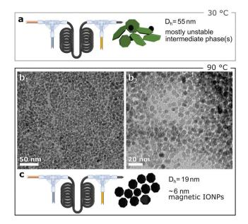
Fig. 4 (a) Schematic of flow synthesis with co-precipitation performed at 30 °C. ( $b_{1-2}$ ) TEM images of IONPs synthesised with co-precipitation performed at 90 °C,  $D_{\text{TEM}} = 6.1 \pm 0.9$  nm. (c) Schematic of flow synthesis with co-precipitation initiated at 90 °C. Fig. S5† shows the particle size distribution. For both temperatures, quenching was performed at 5 s.
