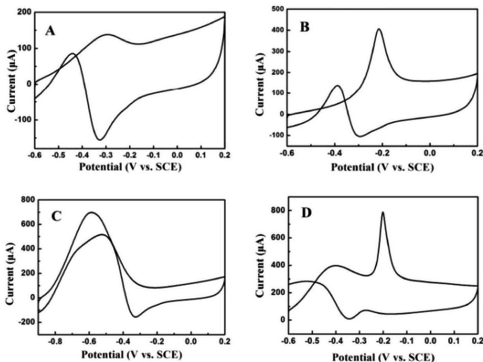
Fig. 9 Cyclic voltammograms recorded for 0.05 M (A) ethanol, (B) ethylene glycol, (C) formic acid and (D) formaldehyde<sup>31</sup> in 1.0 M KOH on the PdNPs/TEG-MWCNT composite modified glassy carbon electrode at a scan rate of  $100 \text{ mV s}^{-1}$ . Adapted with permission from ref. 31, copyright 2018 Elsevier.
