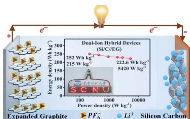
Fig. 7 Schematic representation of the dual-ion hybrid devices<sup>117</sup> fabricated with a silicon–carbon anode and expanded graphite cathode adapted with permission from ref. 117 copyright 2020 Royal Society of Chemistry.
