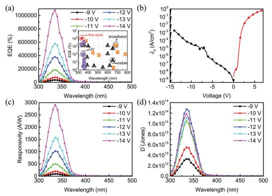
Fig. 2 (a) EQE, (b)  $J_d - V$ , (c) R, and (d)  $D^*$  characteristics of the fabricated UV PM-type OPDs under different applied voltages. The device structure is  $ITO/TAPC: C_{60}(50:1, 80 \text{ nm})/Al(100 \text{ nm})$ . Inset of (a): summary of the peak EQEs of our prepared devices and the reported organic or organic/inorganic photodetectors.
