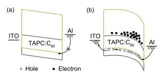
Fig. 3 Energy band structures of the fabricated UV PM-type OPDs at reverse bias under (a) dark and (b) light conditions. The device structure is ITO/TAPC: C<sub>60</sub> (50:1, 80 nm)/Al (100 nm).
