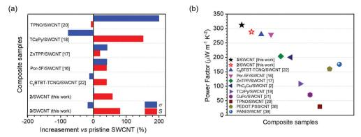
Fig. 4 (a) Increasement of S and  $\sigma$  values of p-type thermoelectric composites made by SWCNT and organic small molecule semiconductors compared with pristine SWCNT. (b) A comparison of the PF values of p-type thermoelectric composites.
