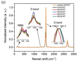
**Fig. 5** Photophysical characterization of pristine SWCNT and OSCs/SWCNT composite films with OSC loading of 50%: (a) UPS spectra, (b) UV-vis-NIR spectra, and (c) Raman spectra.
