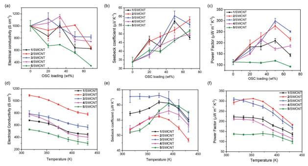
Fig. 3 The  $\sigma$  (a), S (b), PF (c) values of OSC/SWCNT composite films at different OSC loadings. The temperature dependency of the S (d),  $\sigma$  (e), PF (f) values of OSCs/SWCNT composite films at OSC loading of 50%.
