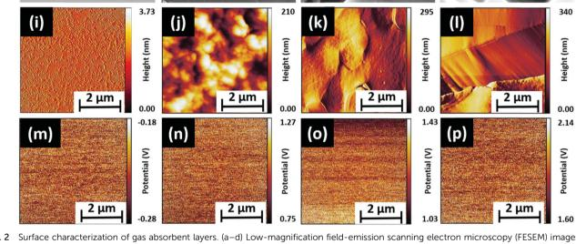
Fig. 2 Surface characterization of gas absorbent layers. (a–d) Low-magnification field-emission scanning electron microscopy (FESEM) images. (e–h) High-magnification FESEM images. (i–l) Atomic force microscopy (AFM) surface topography images. (m–p) Kelvin probe force microscopy (KPFM) images of gas absorbent materials PDVT-10 (M1) (a, e, i, m), HDN4 (M2) (b, f, j, n), HDN6 (M3) (c, g, k, o) and HDN7 (M4) (d, h, l, p).
