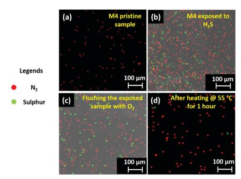
Fig. 6 Surface optical characterization of the M4 material. Energy-dispersive X-ray spectroscopy (EDX) map of (a) a pristine M4 thin film sample, (b) a H<sub>2</sub>S-exposed M4 sample, (c) a H<sub>2</sub>S-exposed M4 sample flushed with O<sub>2</sub> gas, and (d) the complete removal of absorbed H<sub>2</sub>S gas molecules from an M4 sample after heating at 55 °C for 1 hour. Red and green dots represent the presence of N2 and sulfur elements on the surface of the M4 thin film
