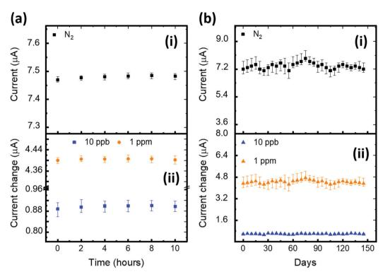
Fig. 5 Stability studies of the D4 OFET  $H_2S$  sensor. (a) Bias stress stability characteristics tested over a period of 10 hours and (b) five-month ambient stability of the D4 OFET sensor toward (i) a  $N_2$  inert atmosphere and (ii) in the presence of 10 ppb and 1 ppm  $H_2S$  gas.
