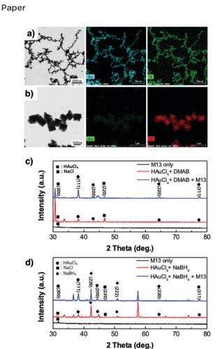
Fig. 3 STEM images and EDS analysis of the virus-templated Au nanowires formed under (a) DMAB and (b) NaBH<sub>4</sub>. XRD spectra of the virus-templated Au nanowires formed under (c) DMAB and (d) NaBH<sub>4</sub>.
