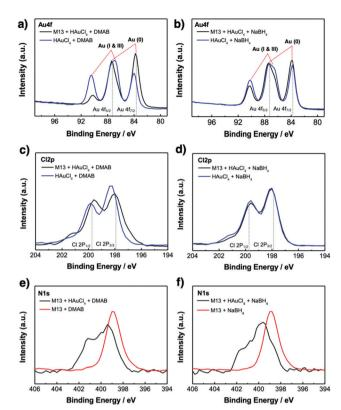
Fig. 4 XPS measurements of Au 4f peaks of the virus-templated Au nanowires made under (a) DMAB or (b) NaBH<sub>4</sub> (blue). (c) Cl 2p peaks of the virus-templated Au nanowires made under (c) DMAB or (d) NaBH<sub>4</sub>. N 1s peaks of the virus-templated Au nanowires made under (e) DMAB and (f) NaBH<sub>4</sub>
