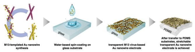
Fig. 1 Schematic illustration of the growth, thin-film fabrication, and transfer of the M13 bacteriophage-templated gold nanowire for stretchable electrode applications.
