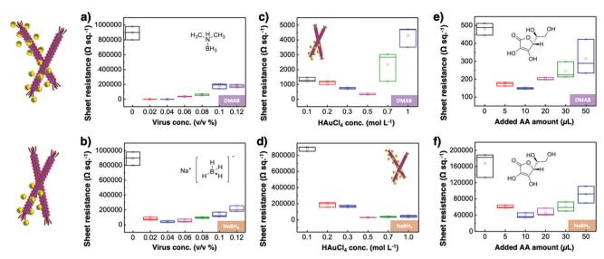
Fig. 2 Sheet resistance according to (a) and (b) virus concentrations, (c) and (d) HAuCl<sub>4</sub> concentrations, and (e) and (f) AA concentrations under DMAB and NaBH<sub>4</sub> reducing agents.
