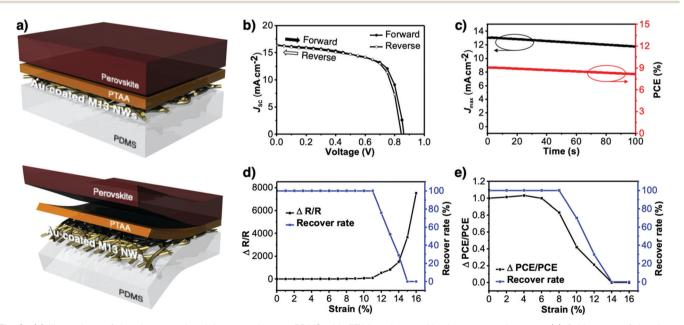
Fig. 6 (a) Illustrations of the virus-templated Au nanowires on PDMS with PTAA and perovskite layers coated on top. (b) J-V curves of the virustemplated Au nanowire-based stretchable PSC under forward and reverse bias. (c) MPPT data of the of the virus-templated Au nanowire-based stretchable PSC. (d) Stretchability data of the virus-templated Au nanowire electrode. (e) Stretchability data of the virus-templated Au nanowire-based PSC.
