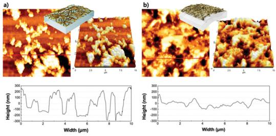
Fig. 5 AFM images ( $10 \times 10 \mu m^2$ ) of M13 bacteriophage-templated Au nanowires on (a) glass, and (b) the surface after transfer to PDMS
