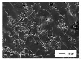
Cross-sectional SEM image of the Na<sub>3</sub>BS<sub>3</sub> glass.
