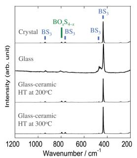
Fig. 4 Raman spectra of Na<sub>3</sub>BS<sub>3</sub> solid electrolytes
