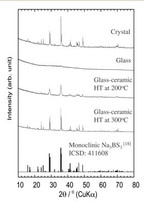
Fig. 1 XRD patterns of Na<sub>3</sub>BS<sub>3</sub> solid electrolytes.
