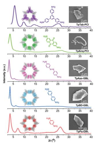
Fig. 2 Examples of experimental PXRD patterns and SEM images of TpPa-GBL, TpBD-GBL, TpAzo-GBL, TpAnq-PCl, and TpTab-PCl COFs.
