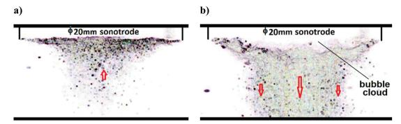
Fig. 1 High speed camera (20k frames per s) snap shot of cavitation underneath a 20 mm diameter sonotrode at: (a) 20 W cm $^{-2}$  and (b) 200 W cm $^{-2}$ . The direction of bubble movement is indicated by the arrows. The bubbles close to the axis centre line of the sonotrode cylinder are faster than those away from the centre line.
