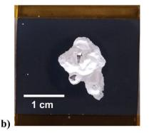
Fig. 2 Images showing the effect of ultrasound on the front side of a QC reject: (a) anode, and (b) cathode sheets. The anode was delaminated in a solution of 0.05 M citric acid; the cathode was delaminated in a solution of 0.1 M NaOH. The sonotrode was 20 mm in diameter, with 120 W cm $^{-2}$  power intensity applied for 3 seconds. Sample size was 3 cm  $\times$  3 cm, placed 2.5 mm away from the sonotrode.
