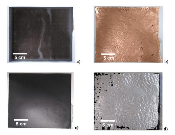
Fig. 4 Images (each 22 cm  $\times$  23 cm) showing: carbon/CMC-SBR/copper electrode (a) before, and (b) after delamination in deionised water (0.05 M citric acid), and NMC/PVDF/aluminium electrode (c) before, and (d) after delamination in 0.1 M NaOH. The delamination was through the 1.5  $\times$  21 cm<sup>2</sup> sonotrode with a power intensity of 70 W cm<sup>-2</sup>, at a sheet feeding speed of 2 cm s<sup>-1</sup>.
