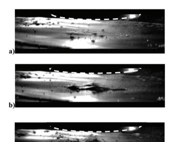
Fig. 3 Images showing snapshots taken from a high speed camera (20k frames per s) during ultrasonic delamination of a carbon/CMC-SBR/copper electrode: (a) 0.01 second after power-on; (b) 0.2 seconds after power-on; (c) 0.5 seconds after power-on. The sonotrode (outlined by the dashed line) was 20 mm in diameter, with 120 W cm<sup>-2</sup> power intensity, at 5 mm from the substrate. The solvent was deionized water.
