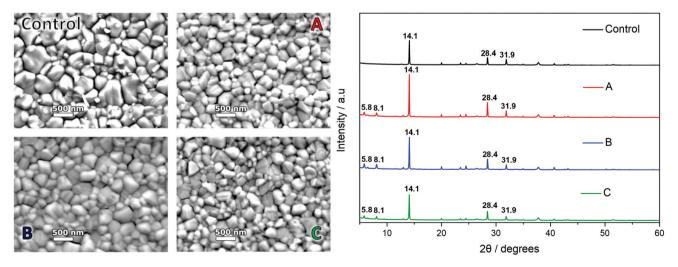
Fig. 6 Top down 30 000× magnification SEM images for candidate solutions A, B, C, and control (DMF/DMSO 80/20 v/v) (left) and XRD scans for candidate solutions A, B, C, and control (DMF/DMSO 80/20 v/v) (right).
