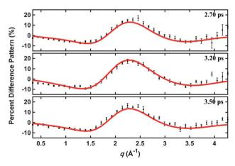
Fig. 5 Experimental and calculated percent difference scattering patterns at several representative delay time points. The experimental results (black dots) are adopted from ref. 14 with  $3\sigma$  error bars and scaled to 100% excitation. Calculated scattering patterns (red lines) are computed using the structural parameters determined with the present method, using the Wigner pool and a computed electronic correction term as described in the text.
