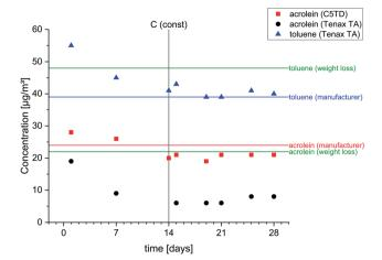
Fig. 2 Concentrations of acrolein and toluene obtained by permeation tubes and active air sampling on Carbograph™ 5TD (C5TD) and Tenax® TA
