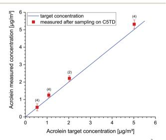
Fig. 4 Acrolein target concentrations in the air of an empty 1 m³ glass test chamber versus acrolein concentration measured after active sampling on CarbographTM 5TD (C5TD). The whiskers show the respective standard deviations, the numbers in brackets indicate the number of repeated measurements. Individual data (target/measured in  $\mu g~m^{-3}$ ): 0.54/0.56  $\pm$  0.21; 1.08/1.25  $\pm$  0.14; 2.03/2.21  $\pm$  0.15; 5.02/5.31  $\pm$  0.25.
