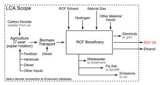
Fig. 9 LCA system boundary diagram, with connections to background LCI database indicated with italics
