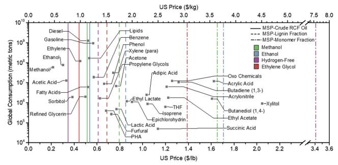
Fig. 8 Minimum RCF oil selling prices with the U.S. price and global consumption of various chemicals for reference. The U.S. Price and Global Consumption data were sourced from a 2016 report by Biddy et al. and are 3–5 year averages. 76 Tabulated data are summarized in Table S34 (ESI†).
