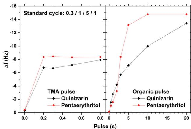
Fig. 2 QCM characterization of growth saturation as a function of pulse durations for Al<sub>2</sub>Qz<sub>3</sub> and Al<sub>4</sub>Pe<sub>3</sub>.
