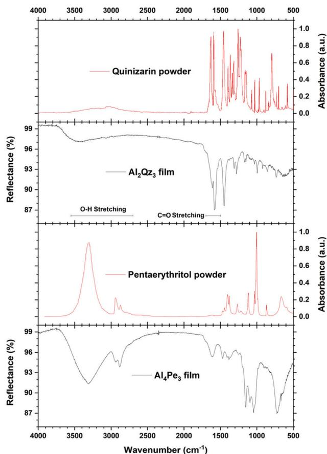
Fig. 5 FTIR data of  $\text{Al}_2\text{Qz}_3$  and  $\text{Al}_4\text{Pe}_3$  films on steel substrates. Quinizarin ( $\text{H}_2\text{Qz}$ ) and pentaerythritol ( $\text{H}_4\text{Pe}$ ) powders in KBr pellets are shown for reference, obtained from the online database Wiley SpectraBase.<sup>28,29</sup>
