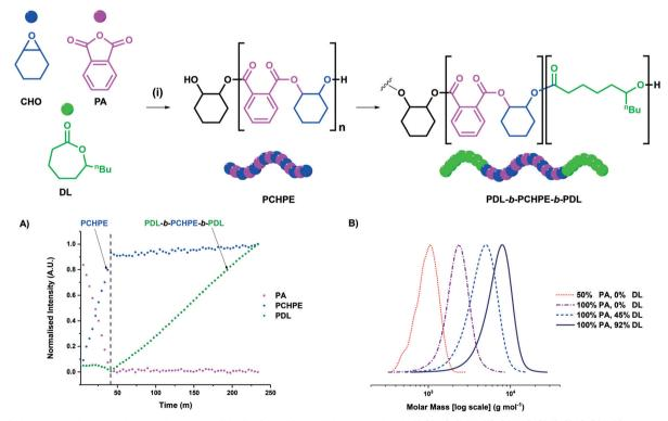
Fig. 3 Switchable polymerization catalysis using PA, CHO and DL utilising complex 1. (i) [Cat]: [PPNCl]: [CHD]: [CHD]: [CHO] = 1:1:10:100: 200:500, T = 100 °C. A) Data from ATR-IR spectroscopy showing the conversion of the different blocks with time. The green series shows formation of PDL, whilst the pink and blue series indicate PA consumption and PCHPE formation, respectively. B) Evolution of polyester molar mass with conversion, from reaction aliquots.
