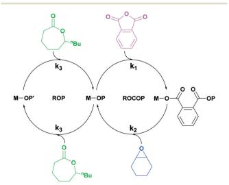
Scheme 1 Illustration of switchable polymerization catalytic cycles using a single catalyst. This method allows for the selective formation of block polymers, commonly in these cycles  $k_1 > k_3$ .<sup>25</sup>
