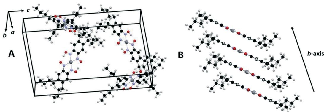
**Fig. 2** Unit cell of [Pt(bqd-dibutyl)<sub>2</sub>] illustrating the herringbone arrangement of molecules in the crystal lattice (A) and slipped stacking of [Pt(bqd-dibutyl)<sub>2</sub>] complexes along the *b*-axis direction (B), generated using Mercury.<sup>29</sup> Pt, N, O, C and H atoms are coloured grey, blue, red, black and light grey respectively.
