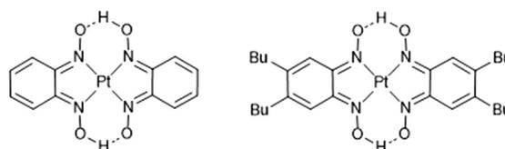
**Fig. 1** Schematic diagrams of [Pt(bqd)<sub>2</sub>] (left) and [Pt(bqd-dibutyl)<sub>2</sub>] (right). The label Bu refers to the *n*-butyl chains.
