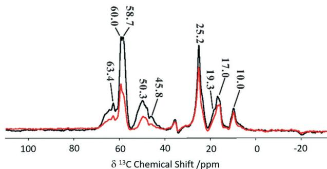
**Fig. 13**  $^{13}\text{C}$  spectra observed with ( $S$ , black) and without ( $S_0$ , red)  $\{^{27}\text{Al}\}$  S-RESPDOR for the trapped products retained in H-ZSM-5 after reaction with methanol for 15 minutes at 573 K. NMR spectra obtained at a MAS rate of  $\nu_r = 10$  kHz. Reprinted (adapted) with permission from ref. 74. Copyright 2017 American Chemical Society.
