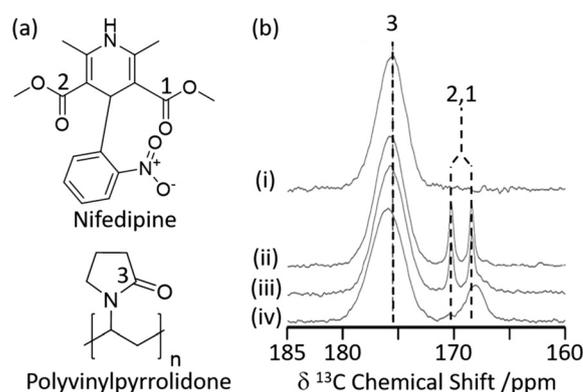
Fig. 2 (a) Chemical structure of nifedipine (NIF) and polyvinylpyrrolidone (PVP). (b)  $^{13}\text{C}$  CP MAS NMR spectra of (i) PVP, a mechanically ground mixture of NIF/PVP/sodium dodecyl sulfate system ground for (ii) 15 min, (iii) 40 min, and (iv) 100 min obtained under MAS at  $\nu_r = 15$  kHz. The spectral assignments are shown in the figure. Reprinted (adapted) with permission from ref. 36. Copyright 2016 American Chemical Society.
