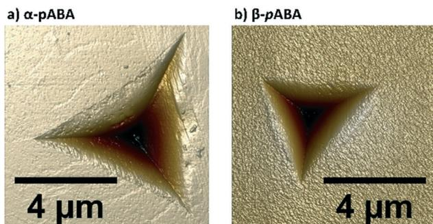
**Fig. 3** Height images (8  $\mu$ m scan size) of indents made on a single crystal of a)  $\alpha$ -*p*ABA and b)  $\beta$ -*p*ABA, acquired using atomic force microscopy (AFM) in PeakForce QNM mode in air.
