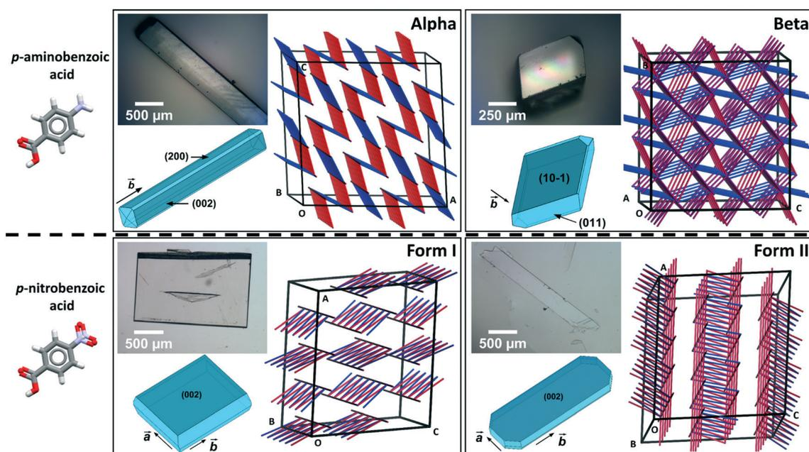
Fig. 1 (Upper) Molecule of *p*ABA, micrographs and face indexing of its alpha and beta polymorph crystals with their respective PBCs. (Lower) Molecule of *p*NBA, micrographs and face indexing of its forms I and II crystals with their respective PBCs. Indented faces are shown in darker blue in the face indexed morphology graph.
