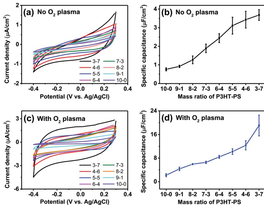
Fig. 6 Electrochemical capacitance evaluation of the structured P3HT films. (a) CV scans ( $100 \text{ mV s}^{-1}$ ) of the P3HT films in the electrochemically-passive region of P3HT. (b) Average  $\pm$  SD of capacitance in  $\mu\text{F cm}^{-2}$  for different P3HT-PS mixing ratios, versus planar. (c) CV scans ( $100 \text{ mV s}^{-1}$ ) of the O<sub>2</sub> plasma-treated P3HT. (d) Calculated capacitance values for plasma-treated samples.
