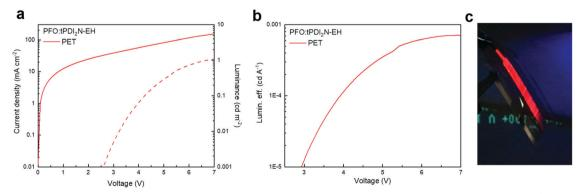
Fig. 5 (a) Current-voltage-luminance characteristics and (b) luminous efficiency (lumin. eff.) versus current density (LE-J, cd A<sup>-1</sup>) of PFO:tPDI<sub>2</sub>N-EH roll-to-roll coated on PET. (c) Photo of electroluminescent of PFO:tPDI<sub>2</sub>N-EH OLEDs on PET.
