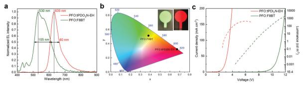
Fig. 4 (a) Normalized electroluminescence (EL) and (b) color coordinates spectra, (c) current-voltage-luminance characteristics of PFO: F8BT (ratio 19:1) and PFO:tPDI2N-EH (ratio 2:18) blends.
