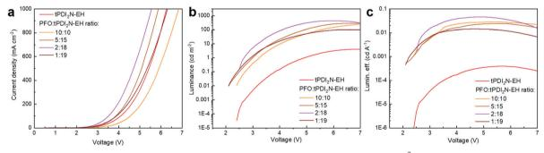
Fig. 3 (a) Current density-voltage (J-V) characteristics, (b) luminance *versus* applied voltage (L-V), cd m<sup>-2</sup> and (c) luminous efficiency (lumin. eff.) *versus* current density (LE-J, cd A<sup>-1</sup>) of PFO:tPDI<sub>2</sub>N-EH OLEDs at selected ratios.
