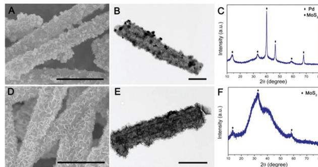
Fig. 4 SEM and TEM images of PPy@MoS<sub>2</sub>@Pd (A and B) and PPy@MoS<sub>2</sub>@Ag (D and E), and (C) XRD patterns of PPy@MoS<sub>2</sub>@Pd (C) and PPy@MoS<sub>2</sub>@Ag (F). Scale bars: 1 μm in (A and D), and 500 nm in (B and E).
