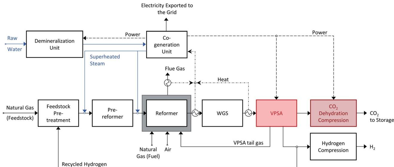
**Scheme 5** Hydrogen production via steam methane reforming with VPSA CO<sub>2</sub> capture and H<sub>2</sub> purification. The VPSA unit replaces the PSA by integrating H<sub>2</sub> purification and CO<sub>2</sub> capture into a single separation unit. The recovered CO<sub>2</sub> is then dehydrated and compressed, while the VPSA tail gas is burnt in the external furnace.
