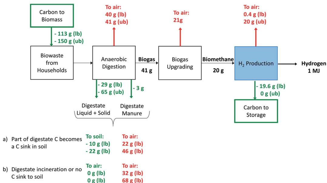
**Scheme 9** Carbon balance of the H<sub>2</sub> production chain based on biowaste, with (lower bound lb) and without CCS (upper bound ub) at the reformer; and with digestate used as fertiliser (a) or digestate being incinerated (b), assuming lower (lb) or upper bounds (ub) of carbon uptake into biomass and carbon sink to soil from digestate.
