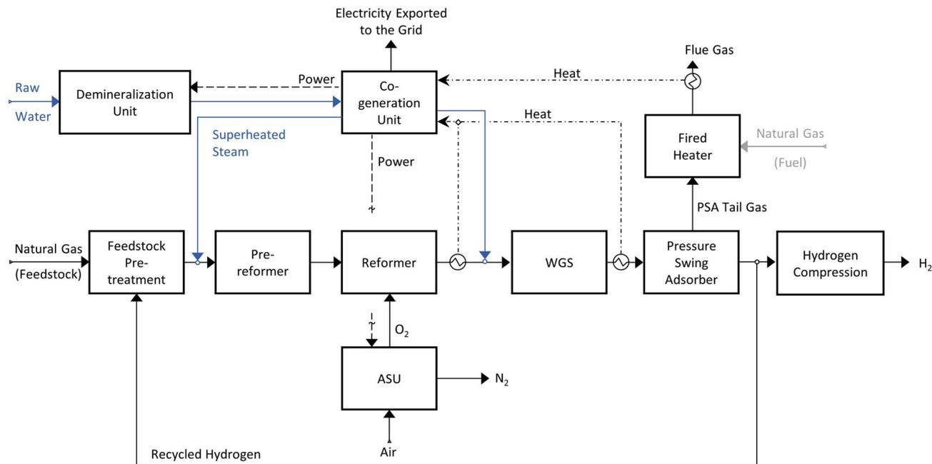
**Scheme 2** Hydrogen production via autothermal reforming; to produce high-purity hydrogen an air separation unit (ASU) is needed. On the contrary to the SMR process, the heat required from the process is internally provided. The PSA tail gas is burnt in a fired heater, and the heat originated by the combustion is used to pre-heat some streams.
