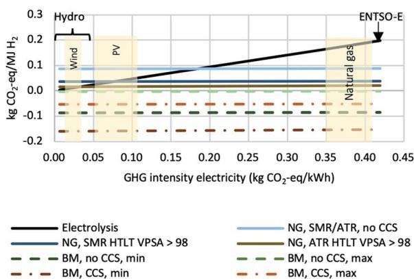
Fig. 7 Life cycle climate change impacts (including infrastructure etc.) for H<sub>2</sub> production via electrolysis or reforming with the configuration "HT + LT, 98% capture rate at CO<sub>2</sub> capture unit" based on natural gas or biomethane. Results are shown in relation to the greenhouse gas load of the input electricity in the foreground system.
