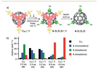
Fig. 4 (a) Cage-templated synthesis of N-methylfulleropyrrolidine trisadducts; (b) relative yields (based on HPLC integration) for unreacted C<sub>60</sub> (black) and Prato adducts 2 (mono, blue), 3 (bis, green) and 4 (tris, red) for control experiment and cage-templated reactions.
