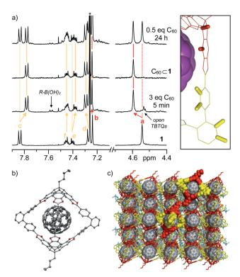
Fig. 3 (a) <sup>1</sup>H-NMR spectra (400 MHz, CDCl<sub>3</sub>, rt) for complexation of 1 with C<sub>60</sub>, (b) ORTEP representation of single-crystal X-ray structure of  $C_{60}\subset 1$  (thermal ellipsoids were set at 50% probability, C= grey, O=red, B = purple, H atoms were omitted for clarity) and (c) packing of  $C_{60} \subset 1$  in the solid state indicating the accessible  $C_{60}$  surface in the three cage windows.
