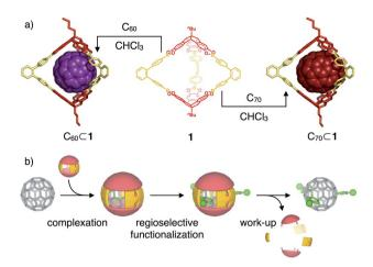
Fig. 1 (a) Supramolecular complexation of fullerenes  $C_{60}$  and  $C_{70}$  within the cavity of covalent organic boronate ester cage 1 (molecular structures of inclusion complexes are derived from semiempirical PM6 modeling); (b) schematical representation for the use of  $C_{60}$ -cage complexes as shadow masks for a regioselective exohedral  $C_{60}$  functionalization.
