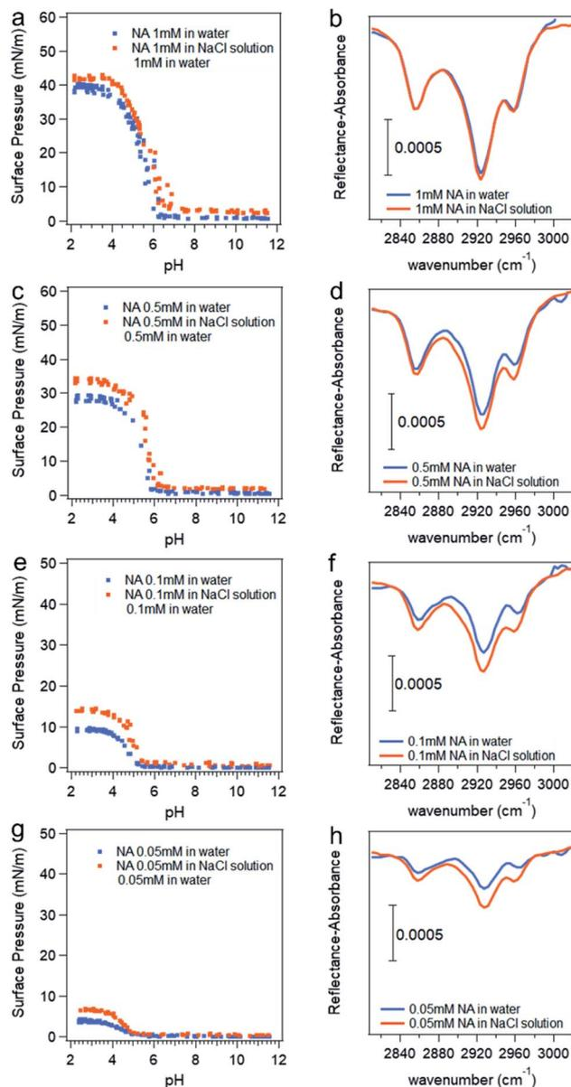
Fig. 5 Surface pressure *versus* pH curves (a, c, e and g) and IRRAS spectra at pH 2 (b, d, f and h) with different nonanoic acid concentration in water compare to in 0.5 M NaCl solution. \*Data points attributed to the “soap effect” in the middle range of the curves shown in Fig. 2 are removed to more clearly show the differences.
