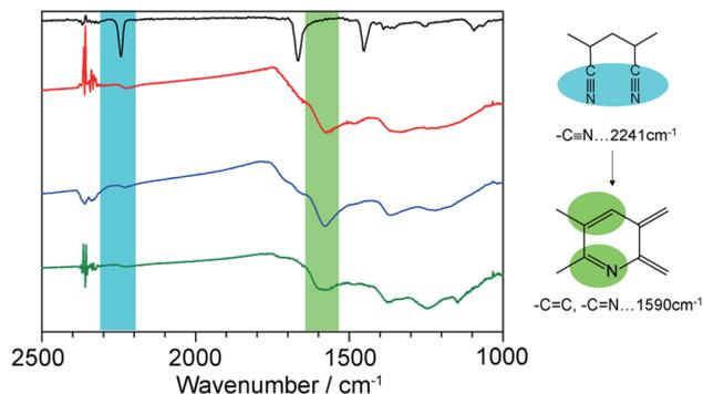
Fig. 4 IR spectra of neat PAN (black), LP liberated from **1a** (red) and **1b** (blue), and LP prepared from neat PAN (green).
