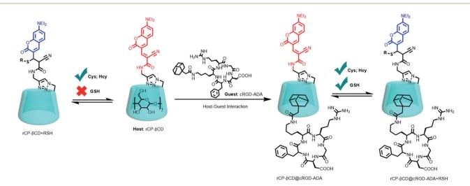
Scheme 1 Construction of rCP-BCD@cRGD-ADA and the reversible Michael addition reactions between rCP-BCD@cRGD-ADA and biothiols.
