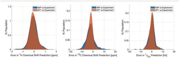
Fig. 4 Distribution of errors for machine learning NMR predictions and DFT calculations when compared to the relevant experimental validation dataset for  $\delta^1$ H (left),  $\delta^{13}$ C (centre) and  ${}^1J_{CH}$  couplings (right). Variance filters applied to IMPRESSION predictions:  $\delta^1$ H = 0.1 ppm (0 of 734 environments removed),  $\delta^{13}$ C = 5 ppm (24 of 457 environments removed),  ${}^1J_{CH}$  = 1 Hz (143 of 608 environments removed).
