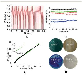
**Fig. 6** Charge–discharge cycles of all iron RFB. (A) 40 charge–discharge cycles at 5 mA cm<sup>-2</sup>. (B) Corresponding CE, EE, VE and volumetric efficiencies. (C) Impedance spectra (green) with simulation (black) after 40 charge–discharge cycles of the membrane. (D) Photographs of the ICEM and Nafion®-112 membranes before and after cycling.
