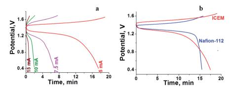
Fig. 5 (a) Overlapping of single charge/discharge cycle recorded at different current densities. (b) Overlapping of single charge/discharge cycle for Nafion®-112 and ICEM at 5 mA cm<sup>-2</sup> current density.
