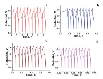
Fig. 4 Initial 20 charge—discharge cycling curves for all iron RFB at different current densities; (a) 5 mA cm $^{-2}$ , (b) 7.5 mA cm $^{-2}$ , (c) 10 mA cm $^{-2}$ , (d) 15 mA cm $^{-2}$ .
