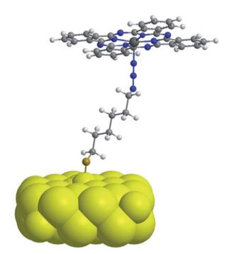
Fig. 6 Simplified schematic illustration of the axial coordination between an immobilized ZnPc molecule on the npAu surface representing the dominant pathway for photoinduced interactions in the ZnPc–npAu hybrid systems. Peripheral substituents of the ZnPc forming covalent connections to the npAu surface through CuAAC were omitted for clarity.
