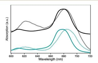
Fig. 5 UV-Vis spectra showing the absorption of the Q-band of the photosensitizer ZnPc with either peripheral propynoxy- (1, H1-7, cyan) or hexynoxy-substituents (2, H2-7, black) in solution (bold line) and when immobilized on a npAu foil (dashed line).
