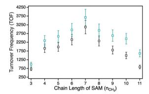
Fig. 4 Photocatalytic  $^1\text{O}_2$  sensitization activities for the hybrids with a systematic variation of the alkyl chain lengths plotted as function of the SAM chain length. Series H1-3–H1-11 with the peripheral propynoxy-functionalized ZnPc derivative 1 is the cyan trace and series H2-3–H2-11 with peripheral hexynoxy-functionalities (ZnPc 2) the black trace.
