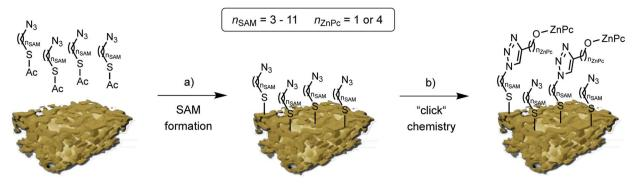
Fig. 2 Schematic representation of the two step npAu powder functionalization: (a) formation of the azide terminated SAM using azidothioates with various alkyl chain lengths, and (b) copper catalyzed azide-alkyne cycloaddition ("click chemistry") to bind the peripherally alkyne-substituted ZnPc derivatives 1 and 2. (npAu modified from [ref. 20]).
