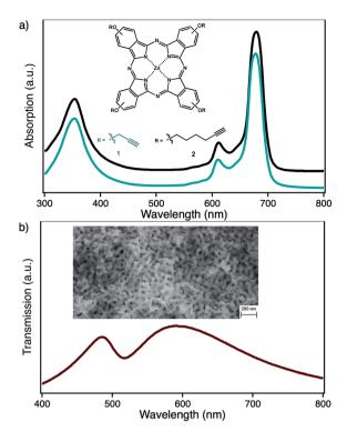
Fig. 1 Structure and corresponding optical spectra for (a) the photosensitizer zinc(III) phthalocyanine with either peripheral propynoxy- (1, cyan) or hexynoxy-substituents (2, black) and (b) nanoporous gold with pore sizes of 40 nm.
