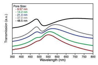
**Fig. 3** UV-Vis transmission spectra of unfunctionalized npAu foils in a DMF surrounding environment after dealloying times of 15 min (red), 30 min (green), 2 h (blue), 8 h (grey) and 72 h (black).
