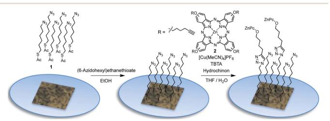
Fig. 4 Schematic representation of the functionalization of the npAu foils: formation of the azide terminated alkanethiol self-assembled monolayer (SAM) in the first step using S-(6-azidohexyl)ethanethioate (1) followed by copper catalyzed azide-alkyne cycloaddition (CuAAC, "click chemistry") to bind the alkyne-substituted ZnPc derivative 2.
