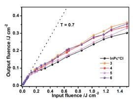
Fig. 4 OL properties of 3-6 in toluene with the initial transmittance (7) of 0.7
