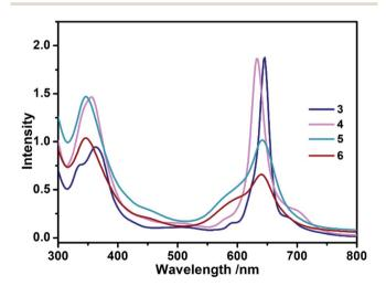
Fig. 1 UV-vis spectra of 3–6 with the concentration of 5.0  $\times$   $10^{-6}~\text{mol}~\text{L}^{-1}$  in toluene.
