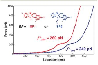
Fig. 7 Representative single molecular force-extension curves of macrocycles incorporating SP1 or SP2 copolymerized with epoxy-COD. Adapted with permission from ref. 218. Copyright 2015 American Chemical Society.
