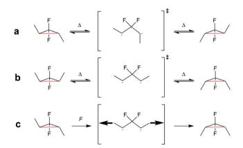
Scheme 23 (a) gDFC E-isomer and (b) Z-isomer thermally ring-open and -close through a disrotatory process via 1,3-diradical transition state. (c) Force leads to the formation and trapping of the 1,3-diradical transition state, which ring-closes to the gDFC Z-isomer once force is removed. $^{123}$
